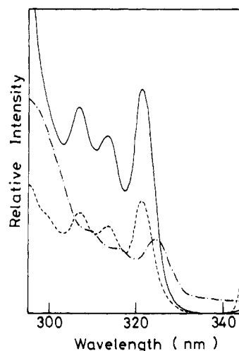
Figure 5. Excitation spectra of Na + -2-NpS - in the presence and absence of PAAH + Cl - at room temperature: (—) Na + -2-NpS - monitored at 345 nm; (---) Na + -2-NpS - /PAAH + Cl - system monitored at 345 nm; (- - -) Na + -2-NpS - /PAAH + Cl - system monitored at 400 nm.
